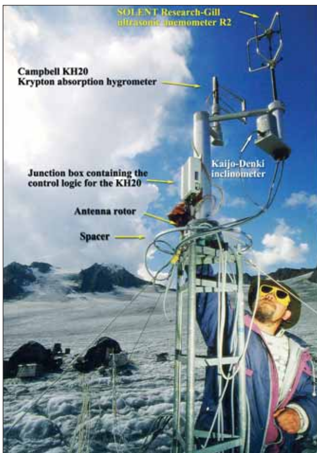
Figure 2: System for eddy correlation measurements, which is mounted on a 2 m tower and run continuously during 5 day periods in August 1998 and 2000, respectively, at Vernagtferner (Oetztal Alps, Austria) at an elevation of 3000 m a.s.l. The glaciologist in Markus Weber, the author. (Photo by Jan Greune)
