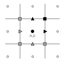
Figure 3.1: Grid variables in hyper are referenced by the abstract cell-centered index to the left and down in 2D (analogously in 3D). In the figure, index (i, j) is used to reference the variables in black. The variables in grey—although contained in the pictured cell—are not referenced by the (i, j) index.
