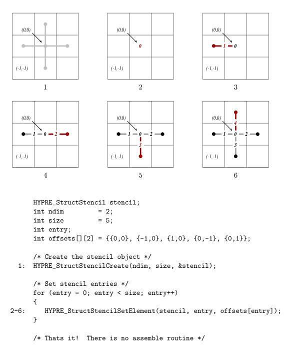
Figure 2.5: Code for setting up the stencil in Figure 2.4.
