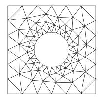
Figure 4.1: Example of an unstructured mesh.
