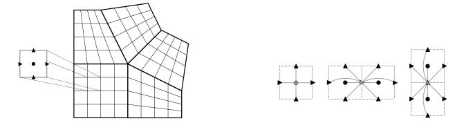
Figure 3.2: Example of a block-structured grid with five logically-rectangular blocks and three variables types: cell-centered, x-face, and y-face. Discretization stencils for the cell-centered (left), x-face (middle), and y-face (right) variables are also pictured.
